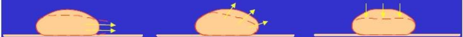
(i) Geotextile skin rupture
